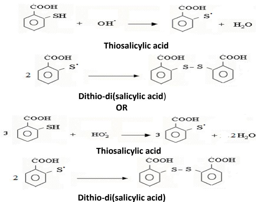
Figure 1: Photo-degradation of Thiosalicylic Acid by Fenton Reagent
